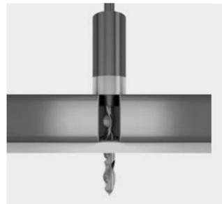
Drilling with drilling jig
