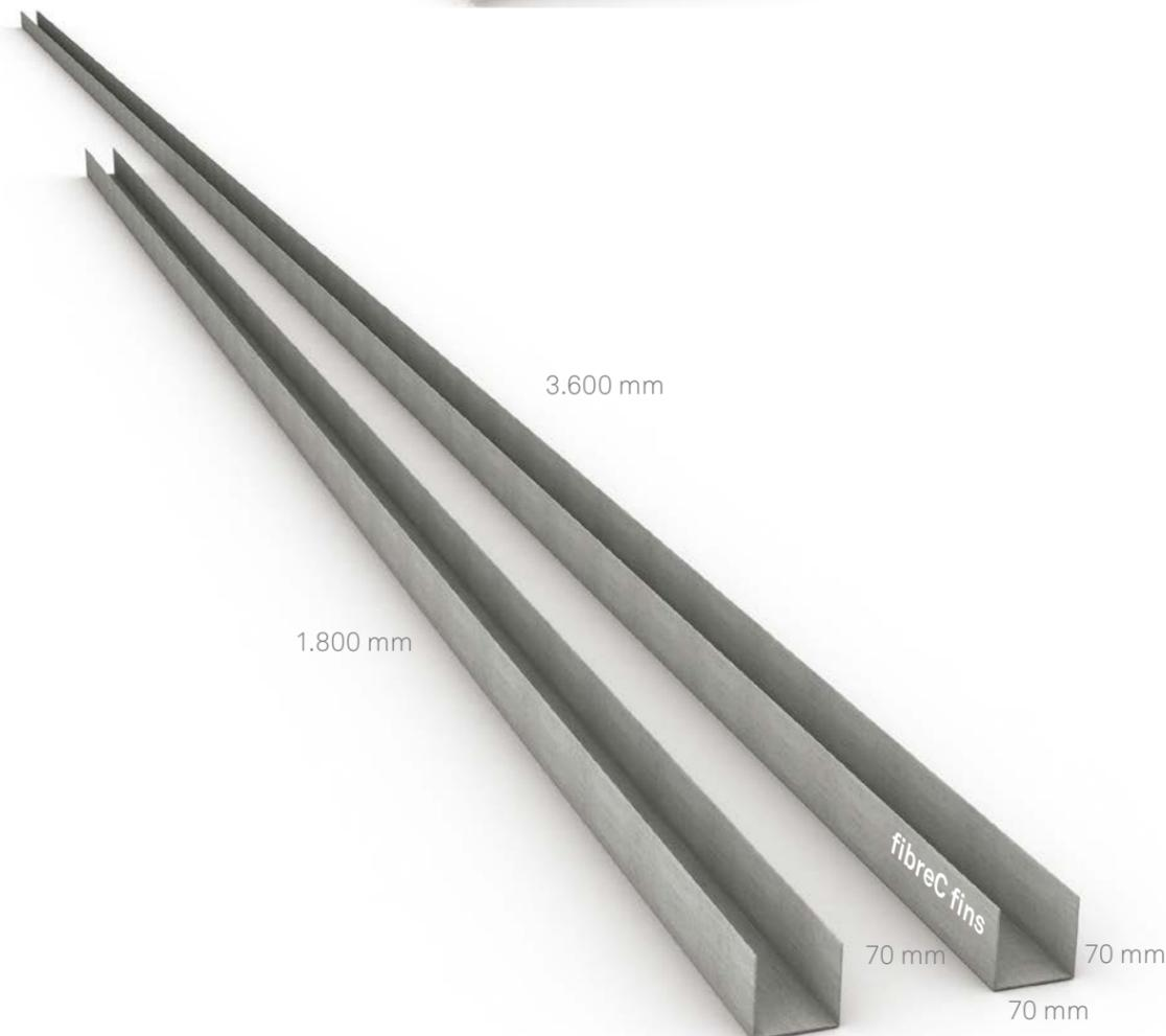
**fibreC fins** are mould elements with U-shaped cross-section in 70 x 70 mm format. fibreC fins are available in 12 colours, 2 surfaces apiece. fibreC fins are popularly used as lean concrete slats for facades, for the purpose of providing large window areas with permanent sun protection or providing the building casing with creative design elements. The geometric shape of the fibreC fins allows for special light effects in interiors when there is daylight outside.
