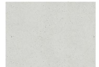
Small air bubbles and porosity are possible: data sheet on exposed concrete 02/2004 (Publ.:BDZ/DBV)
