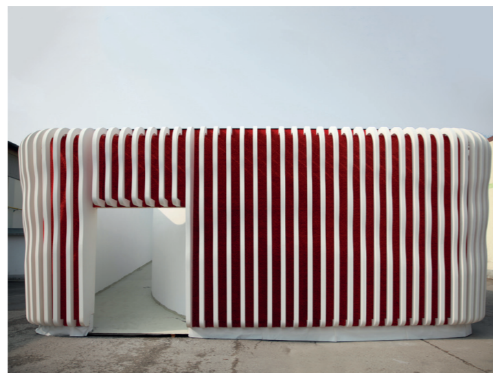
Pavilion enveloped with wavy concrete slats
